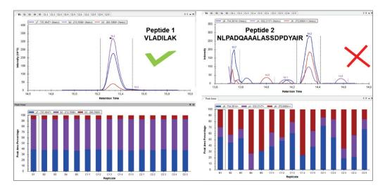
Figure V-1 – Example of chromatographic peaks obtained for two peptides in fifteen different samples (histograms). The different transitions are represented with different colors (violet, blue and brown). Histograms represent the percentage of contribution of each transition to the total area of the peak.
